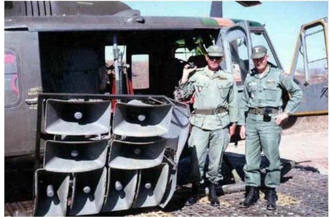
Loudspeakers mounted on a Huey helicopter used for playing the Wandering Soul tape.
